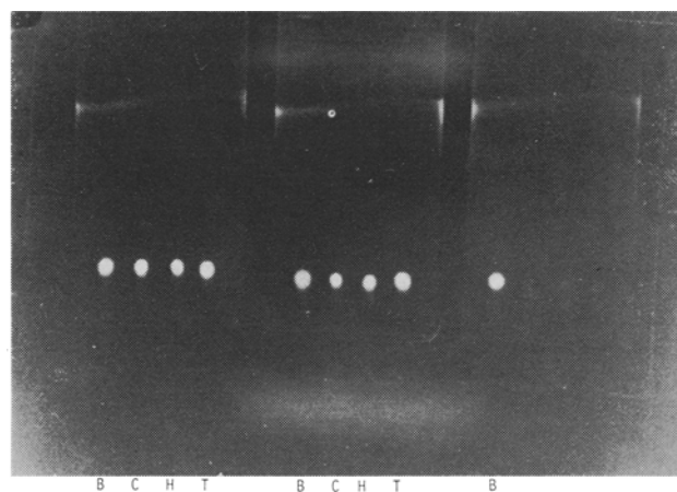
FIG. 1. Composite picture of aflatoxin B 1 standard solutions (5 µg/mL) spotted on TLC strips. Strips represent solutions at 3 storage levels. Each spot contains 5 µL of standard solution: b = benzene, c = cyclohexane, h = heptane, t = toluene. First TLC strips on left with 4 spots are standards after 0 time of storage. Second or middle TLC strip with 4 spots are standard after 6 months storage in the dark and at ambient temperature. Third, TLC strip on right with lone spot is that of standards after 3 months storage in open laboratory light and at ambient temperature. Development was made with diethyl ether/methanol/water (96:3:1) for 10 min. Detection was made with long-wave UV light.
